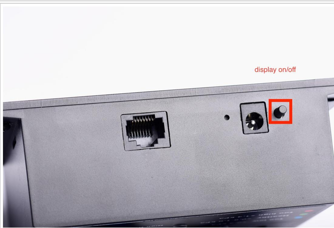
On/off switch for display lighting
