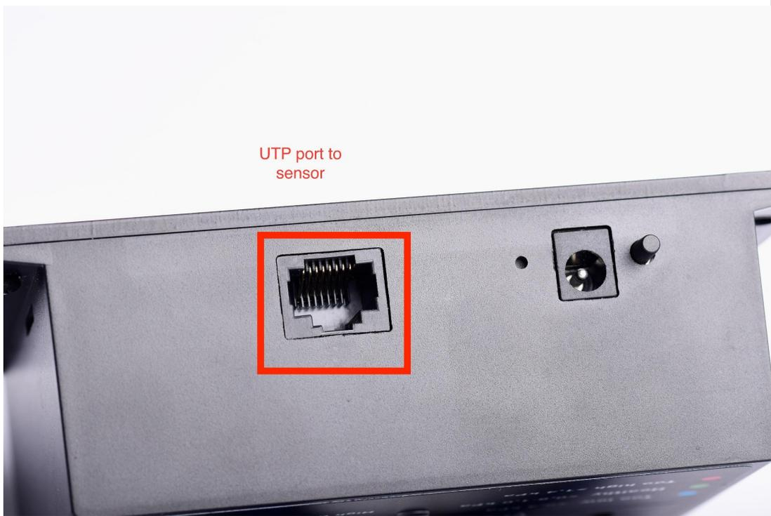
UTP port that connects the Display unit to the sensor unit
