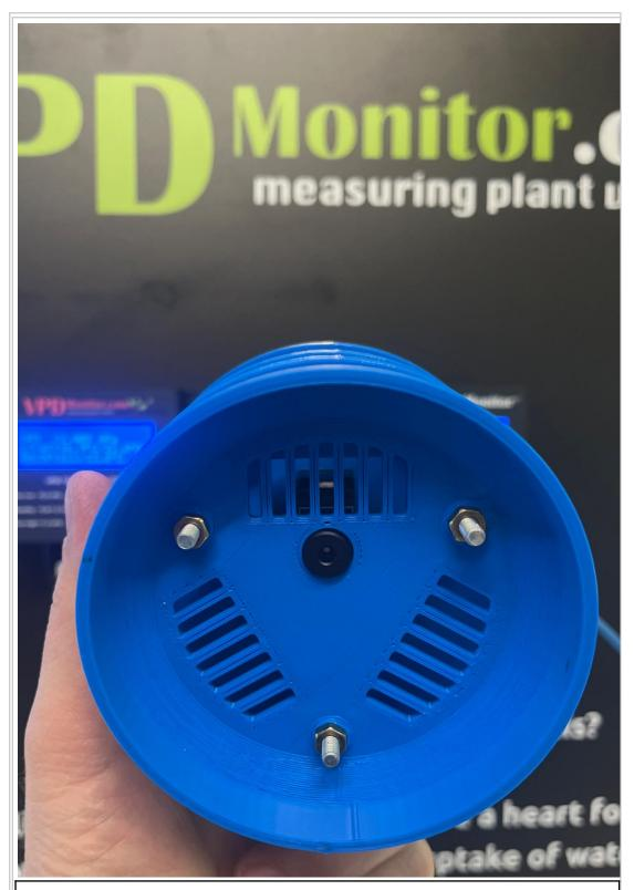
Bottom view of the sensor unit with the LT sensor visible
